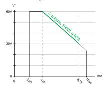
Output voltage vs output current for 4 outputs with symmetrical load  $Vf_{typ}$  is 57V, LED current ranges from 200mA - 1050mA
