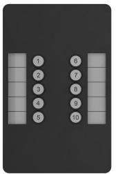
The front panel interface contains 10 10Scene buttons, these have dual colour LEDs used to indicate when a Scene has been stored to a button and when a Scene is active. When a button LED is Blue this indicates a Scene has been stored, but is not active, when in Red this indicates the Scene is active.
